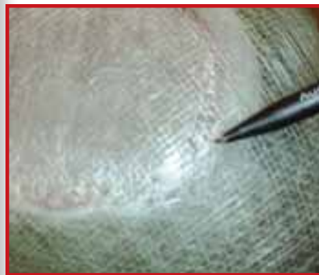
Left, below: Damaged area to be repaired caused by seat scraping on track. Damage extends all the way through the seat.
