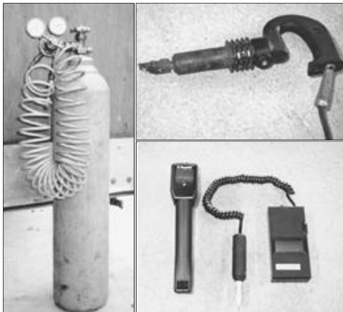
Left: Nitrogen is used to fill tires because it expands less than air. Top: This device is recommended for sipping the tires to get lasting usage. Bottom: These small tools are easily portable and allow you to test the tire temperature anywhere in the pits or on the grid.
