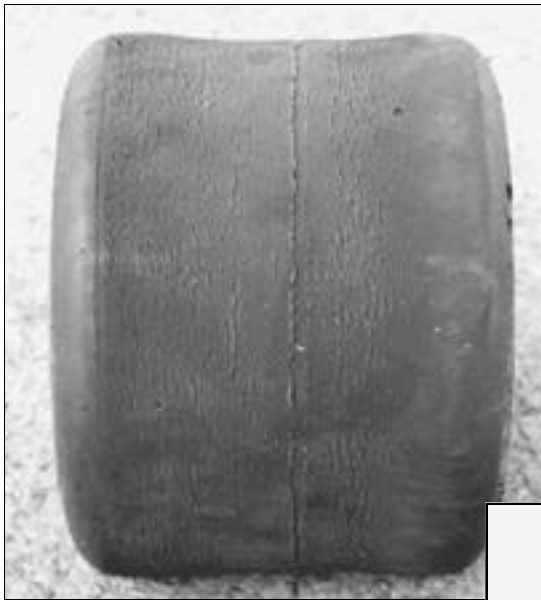
Heavy feathering occurs when a tire has too soft of a compound for the track conditions. Notice the ripple effect that has occurred.
