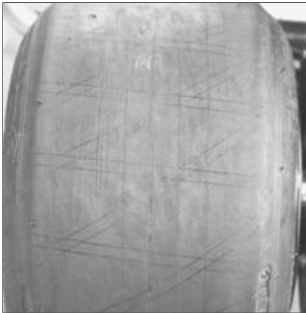
This is a rear tire sipping pattern suggested for use in this application of dirt racing.
