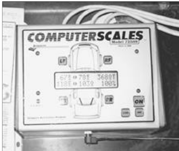
This view gives you a readout of the kart's weight distribution.
