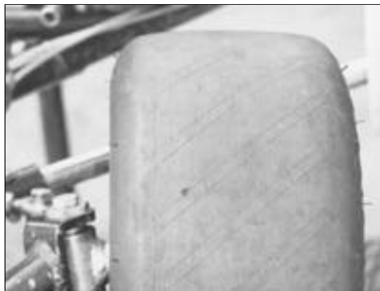
Another example of sipping, this one on the front tire.
