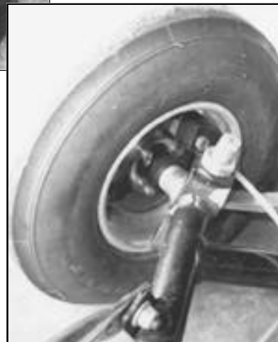
Hegar front brakes are assembled inside the wheel.
