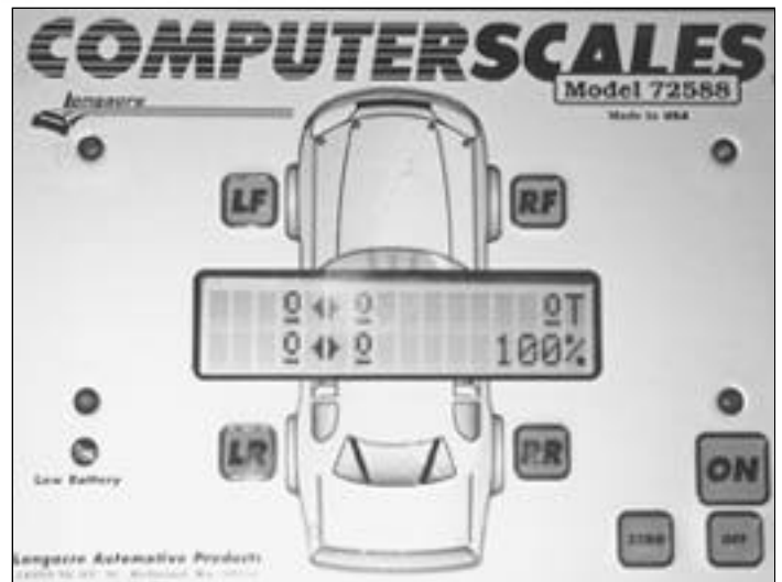
Top: This chassis scale was designed specifically for karts and is giving a reading without a kart on the scale.
